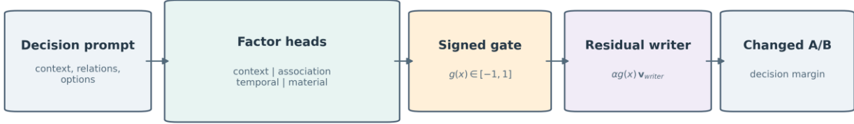
Figure 1. GraftLoyal runtime mechanism. Frozen factor heads estimate the semantic conditions for loyalty, a signed competition-aware gate determines direction and strength, and a residual writer changes the A/B decision margin.
